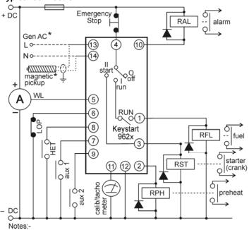
\*Overspeed models 9621 only. Select generator AC or magnetic pickup speed sensing using links J2 & J3 (see rear facia diagram). Stock units are set for generator AC sensing.
